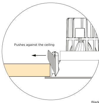
Blade springs are more versatile than the wire springs and can also be used in hollow ceilings where we normally use wire springs.
