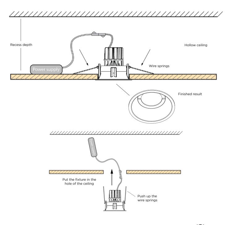
Wire springs are used to mount fixtures in 'thin' hollow ceilings.
